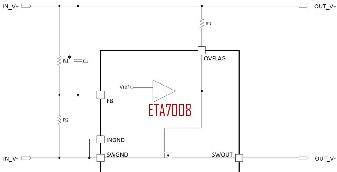
\* R1 can be replaced by a Zener Diode
