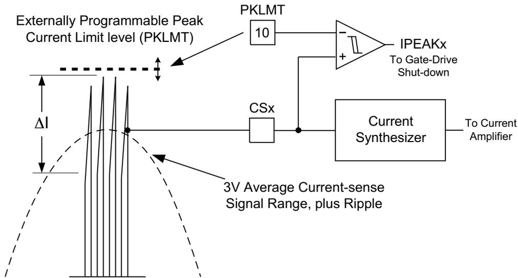
Figure 20. Externally Programmable Peak Current Limit
