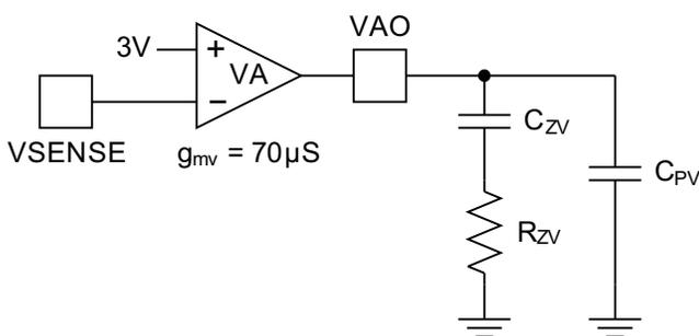
**Figure 23. Voltage Error Amplifier With Type II Compensation**
