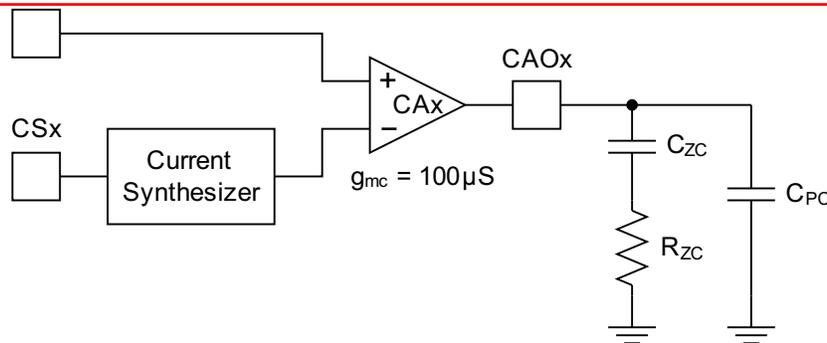
Figure 22. Current Error Amplifier With Type II Compensation
