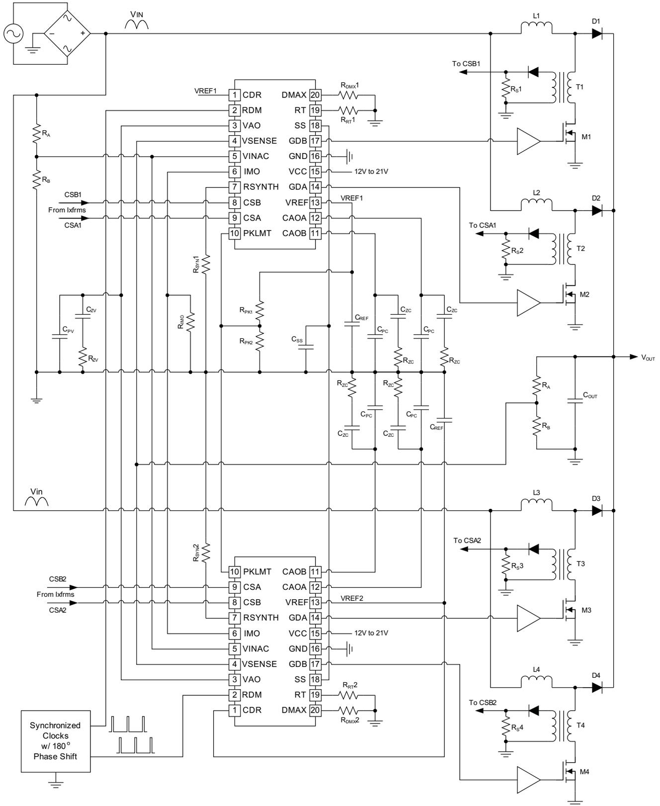
Figure 18. Simplified Four-Phase Application Diagram Using Two UCC28070
